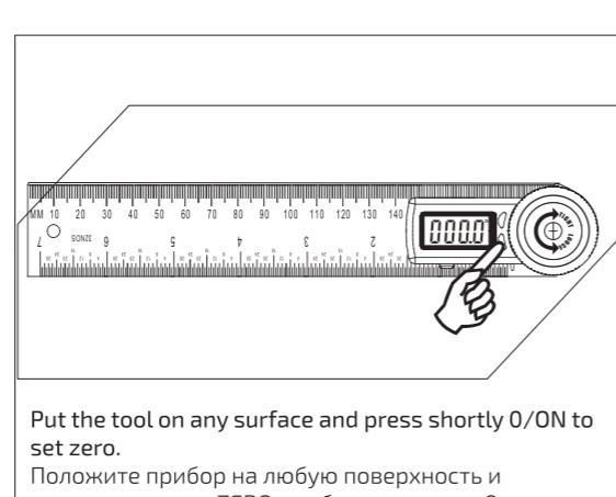
Put the tool on any surface and press shortly 0/ON to set zero.
