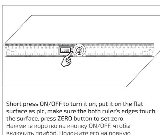
Short press ON/OFF to turn it on, put it on the flat surface as pic, make sure the both ruler's edges touch the surface, press ZERO button to set zero.
