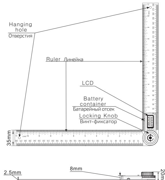
**ON/OFF** Short press ON/OFF to turn on the device. Short press ON/OFF to shut off the LCD. Long press ON/OFF for more than 3 seconds to shut off the whole system. Automatically shut off function in 6 min. Move the scale to turn on the device when at off LCD status.
